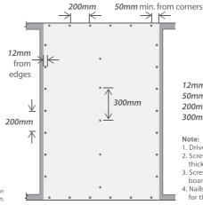
12mm min. from edge 50mm min. from corner 200mm centres max. at sheet perimeter 300mm centres max, elsewhere
